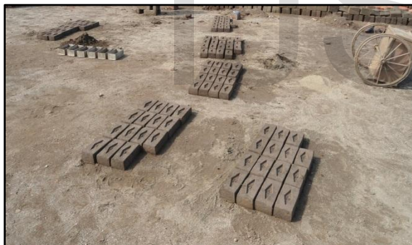
Fig. 3 Drying raw bricks before baking
