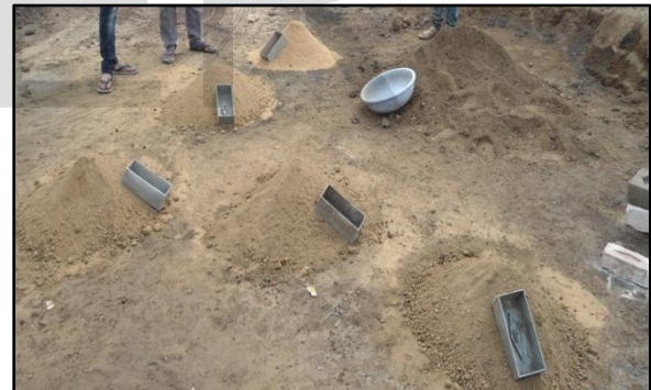
Fig. 1 Mixtures of CSP and soil for making bricks
