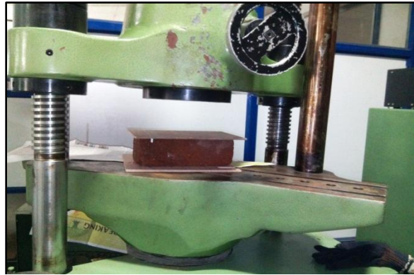
Fig. 6 Specimen of sample 1 during compression test
