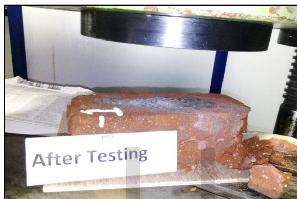
Fig. 7 Specimen of sample 1 after compression test
